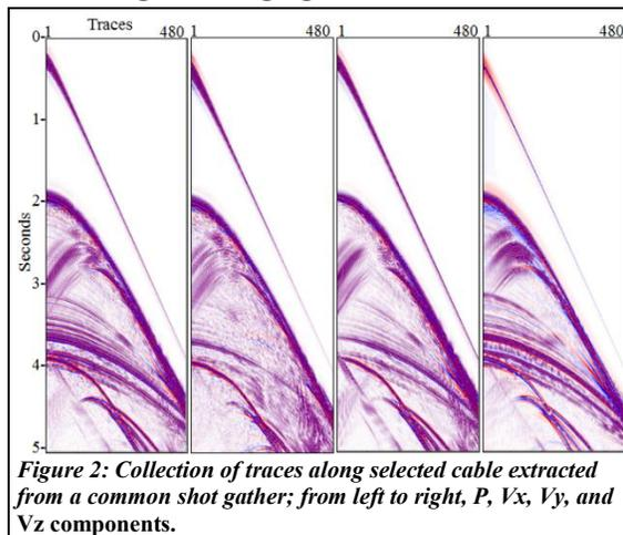
Figure 2: Collection of traces along selected cable extracted from a common shot gather; from left to right, P, Vx, Vy, and Vz components.
