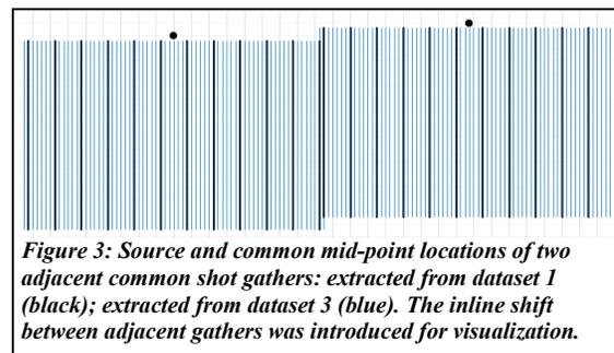
Figure 3: Source and common mid-point locations of two adjacent common shot gathers: extracted from dataset 1 (black); extracted from dataset 3 (blue). The inline shift between adjacent gathers was introduced for visualization.
